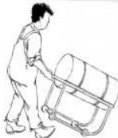
Figure 24: Drum handlers are available for most sizes of drums. This allows their convenient tilting and lifting.
